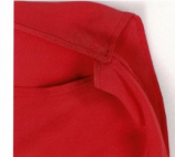
30.7. The RS of the left shoulder. The point of the back body piece is stitched over the front.
