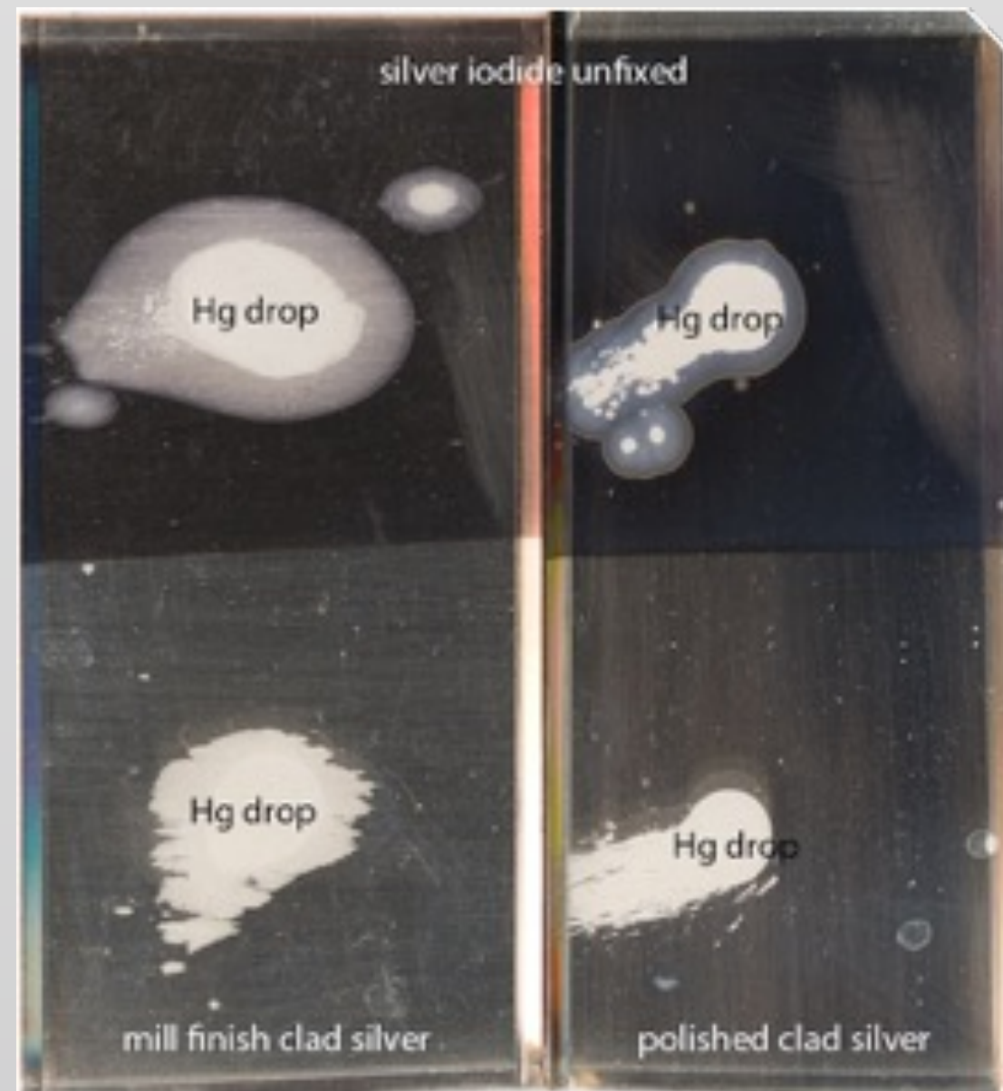
DagTest 11-21-2011. Mercury droplet test.
